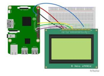
OLED Pin #1 to Raspberry Pi GND
