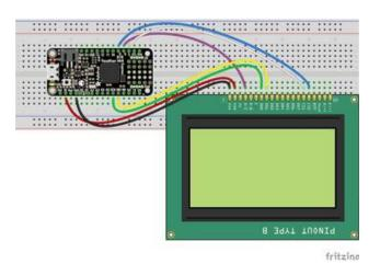
OLED Pin #1 to Microcontroller GND
