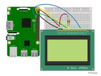
OLED Pin #1 to Raspberry Pi GND
