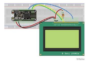
OLED Pin #1 to Microcontroller GND
