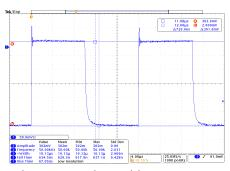
50 kHz, 10 μs Pulse Width, 60 A Output
